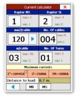
The Raptor Current Calculator is included as standard in the Raptor HH console and can also be installed on a PC. It is a simple to use yet sophisticated tool that allows the user to quickly define the Raptor configuration and the number and type of cables required as minimum to successfully accomplish a specific high current job, even before leaving the office.
