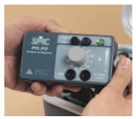
the PTE range from 10 to 120V with a maximum current of 0.3A
