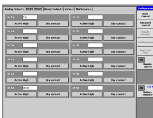
Furthermore, each voltage amplifier can be switched to current mode by a simple touch on the configuration screen. This feature allows, for example, to convert a MENTOR 12 3v3i (3 voltage + 3 current channels) to a six-current test set when the need for testing three-phase differential relay arises. Low Level Outputs and superimposed harmonics for every source can also be activated in this control.
