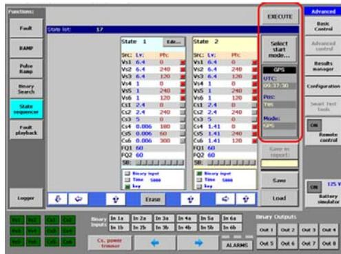
**MENTOR-GPS/IRIG-B:** Certain kind of test requires the setup of two or more MENTOR 12 units (or one MENTOR 12 and other test set) separated on different locations and synchronized with each other. In this case a very high precision reference clock is necessary, in order to obtain the required timing to trigger the state sequencer or the reproduction of Fault playback (COMTRADE files) on separate units.
