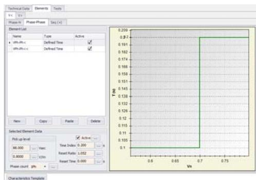
Set of Voltages Modules to test the operation of protective devices with functions 27, 47 and 59. It includes the following modules to test the operation values of voltage relays:
