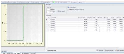
The frequency module is used to test the operation of protective devices with frequency dependent functions. This includes functions of frequency, under and over frequency, Hz/s element (rate of change of frequency), and V/Hz protection (overflux or overexcitation element)
