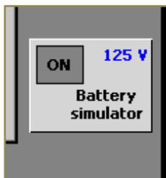
**Battery Simulator:** The MENTOR 12 has a built-in battery simulator up to 250 Vdc, which must be used to supply the relays being tested and which require an auxiliary power supply. The Battery Simulator control is available in all the accessible function screens.
