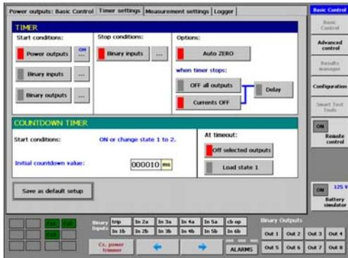
**Timer Settings:** Timer start and stop conditions can be quickly adjusted to the test needs. The timer can be programmed to start by the status changes in the Power Outputs, by the action of a Binary Input combination, or by the status change of any Binary Output. Timer stops by the trip action at the Binary Input logic, which setting is straightforward selected. After the stop of the timer, voltage and/or current outputs can be immediately switched off or delayed to simulate switch time.
