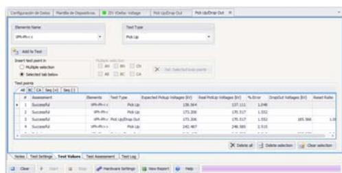
**Test List:** Click Sequence and Pick up/Drop out tests can be attached to any of the two modules.
