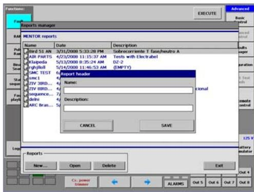
**Results Manager:** The Results Manager allows saving both the test results and configuration of Advanced test functions, so that they can be repeated as desired. Results are saved in a USB pendrive.
