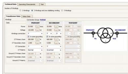
**TRANSFORMER DIFFERENTIAL 87T:** Designed for testing numerical relays for differential protection of transformers. The module's functionality is distributed in the following sections:
