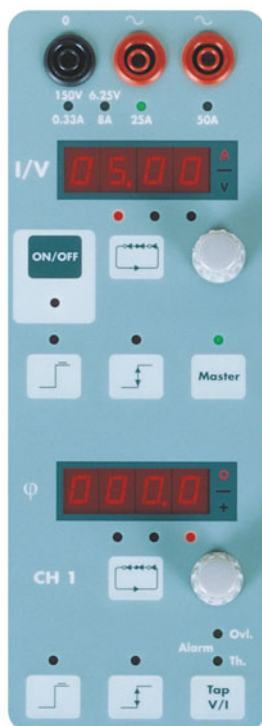
Canal de courant/tension
